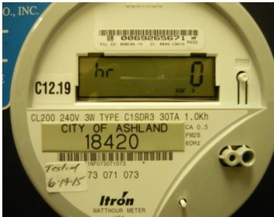
**Screen 3: hr** This screen shows the Kilowatt hours received from the customer. **This is the excess solar generated power that is not being used by the customer, is going onto the City of Ashland grid, and the customer is credited for.**
