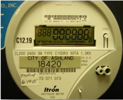
**Screen 1:** This is the LCD test screen. All numbers and letters will be illuminated to show that the LCD is working correctly.
