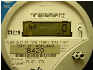
**Screen 2: hd** This screen shows the Kilowatt hours delivered to the customer from the City of Ashland Electric Utility. This is the power that the customer is billed for.
